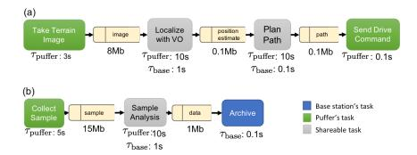
Figure 2: PUFFERs software network.
