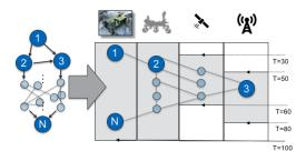
Figure 1: Illustrative MOSAIC scenario. A set of processing and data-driven tasks (left as dependency graph) must be mapped to multiple assets with heterogeneous computing, communication, and energy capacities. Each asset is also available over a fixed time window due to terrain effects or orbital parameters. The goal is to compute all the required tasks as quickly as possible.
