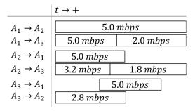
Figure 3: Contact graph for 3 agents showing connectivity time windows and bandwidths available.
