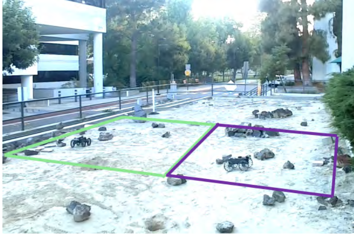
Fig. 2: Testing the proposed algorithm at the Moon yard at JPL. The yard is cluttered with rocks, craters and uneven surfaces to resemble lunar surface. The violet and green rectangles represent the map partitions output by our algorithm corresponding to the two robots.
