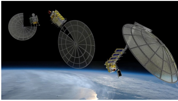
Fig. 9: Artist's representation of Made In Space's Archinaut spacecraft 3D-printing and assembling satellite reflectors in space. (image credit: Made In Space 61 )
